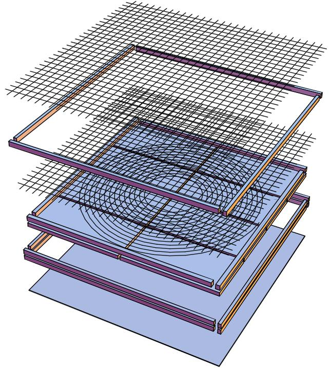
Figure 2: Exploded view of the  $2 \times 2 \text{ m}$  test version of the proposed collector. From bottom to top: bottom cover, wooden side bars, insulation layer for bottom and sides on which the tube in spiral, plastic foil with chicken wire, more wooden side bars, upper plastic foil with chicken wire
