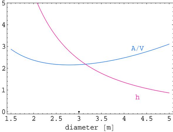
Figure 3: *Compromise between diameter and height for a cylindrical heat store with 17m<sup>3</sup> water. On the horizontal axis is the diameter, the red line gives the corresponding height, the blue line gives the relative area A/V. At h = d = 2.70 m the ratio A/V is minimal. Note that one can chose a much larger diameter and lower height in order to reduce the hydrostatic pressure without increasing much the ration A/V*
